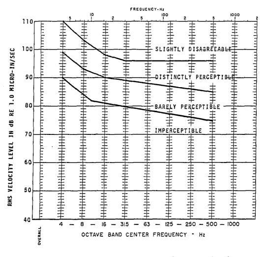
THE CHART INDICATES THE RANGE OF RESPONSE Level for seated or standing persons subjected to vertical mechanical vibration
