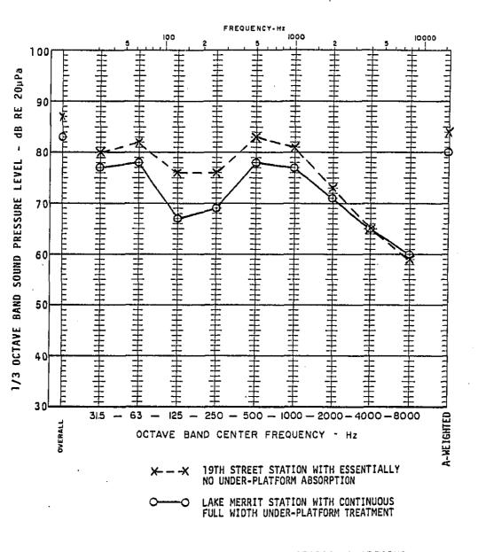
FIGURE 38 NOISE LEVELS ON BART UNDERGROUND STATION PLATFORMS WITH TRAINS PASSING THROUGH AT A CONSTANT SPEED OF 20 MPH
